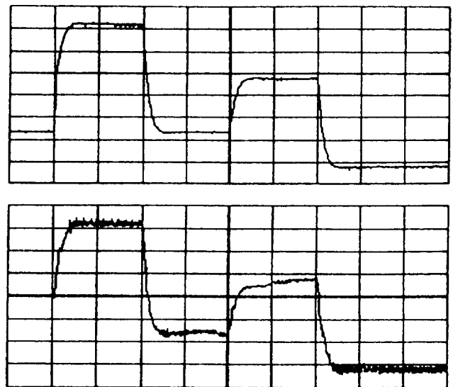
Figure 4: Response of model (top trace) and motor (bottom trace) to reference step of 800 rpm at 0.5 sec., step to -400 rpm at 1.5 sec., step to 200 rpm at 2.5 sec., step to -800 rpm at 3.5 sec., (0.5 s/div)
